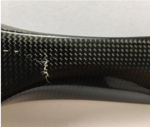
Unacceptable propeller crack
