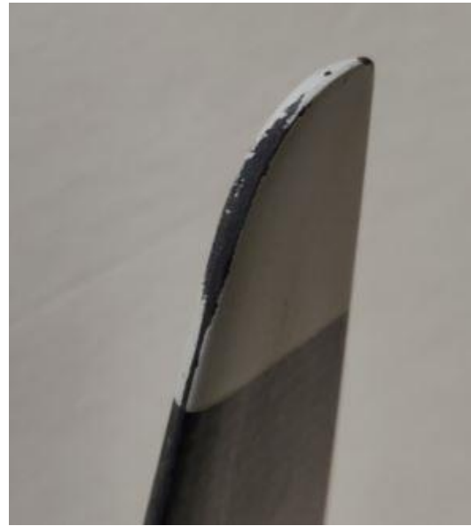
Acceptable paint scratches
