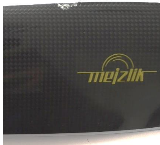
Unacceptable propeller crack
